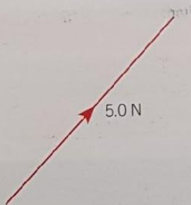
▲ Figure 2 Representing a vector quantity, in this example a force of 5.0\text{ N}
