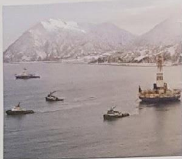
▲ Figure 1 Tugboats towing an oil platform
